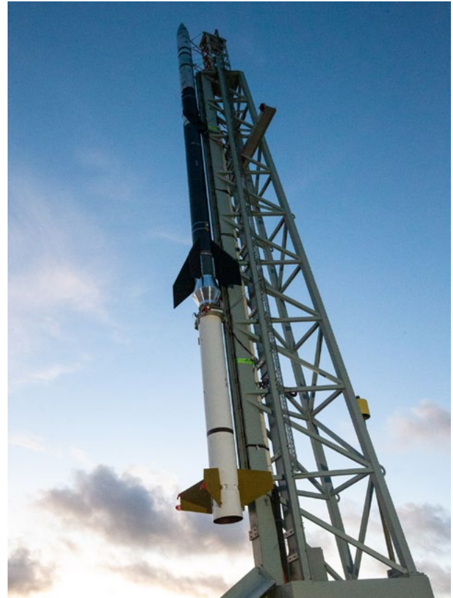
XQC ready to fly on a Terrier-Black Brant Sounding Rocket Credit: Wallops Imaging Lab.
