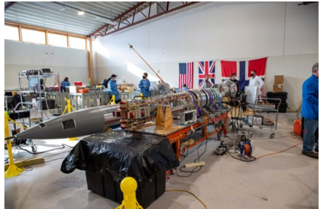
Endurance payload during buildup in Svalbard. Credit: Brian Bonsteel/NASA Wallops Imaging Lab.
